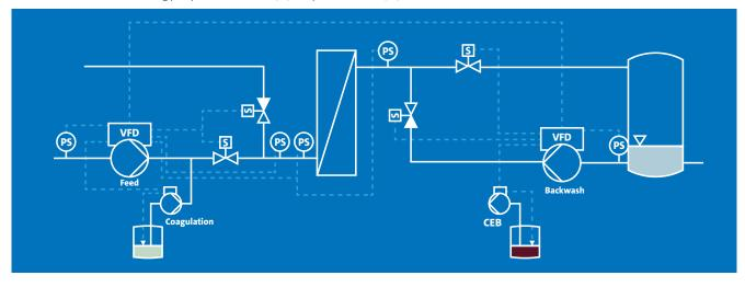
An example of the integration and control of a decentralised ultrafiltration with Grundfos isOLUTIONS. E-Pump recommendations for the system are either NBE, NKE or CRE with a DDA dosing pump with flow sensor (FS) and pressure sensor (PS).
